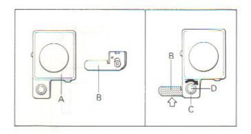
In drive lace knitting, use P Carriage "A" without P Presser "B". In pile knitting, use P Carriage "A"-with P Presser "B" attached. Place P Presser "B" underneath Arm "C" and secure with fastening screw "D".
