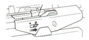
7 Exchange waste yarn for pile yarn in main Yarn Feeder.
