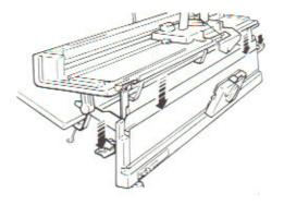
Lower Ribber Needle Bed to the middle position by depressing Drop Lever (marked red) once.
