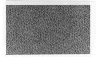
Perforated area of Punch Card knits Stockinet and non-perforated area leaves a loop of yarn in needle hooks.
